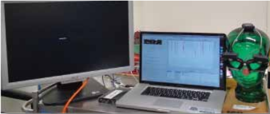
Video-based system to study eye movements might become the way in the future. On the left is a large screen displaying target jumps for saccade, in the middle is the laptop computer containing the software to drive the entire system, and on the right lightweight video goggles capable of capturing eye movements from both eyes.
